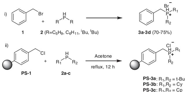
**Scheme 1.** Syntheses of tertiaryphosphine salts **3a–3d** and polymer-supported ligands **PS-3a–c**.
