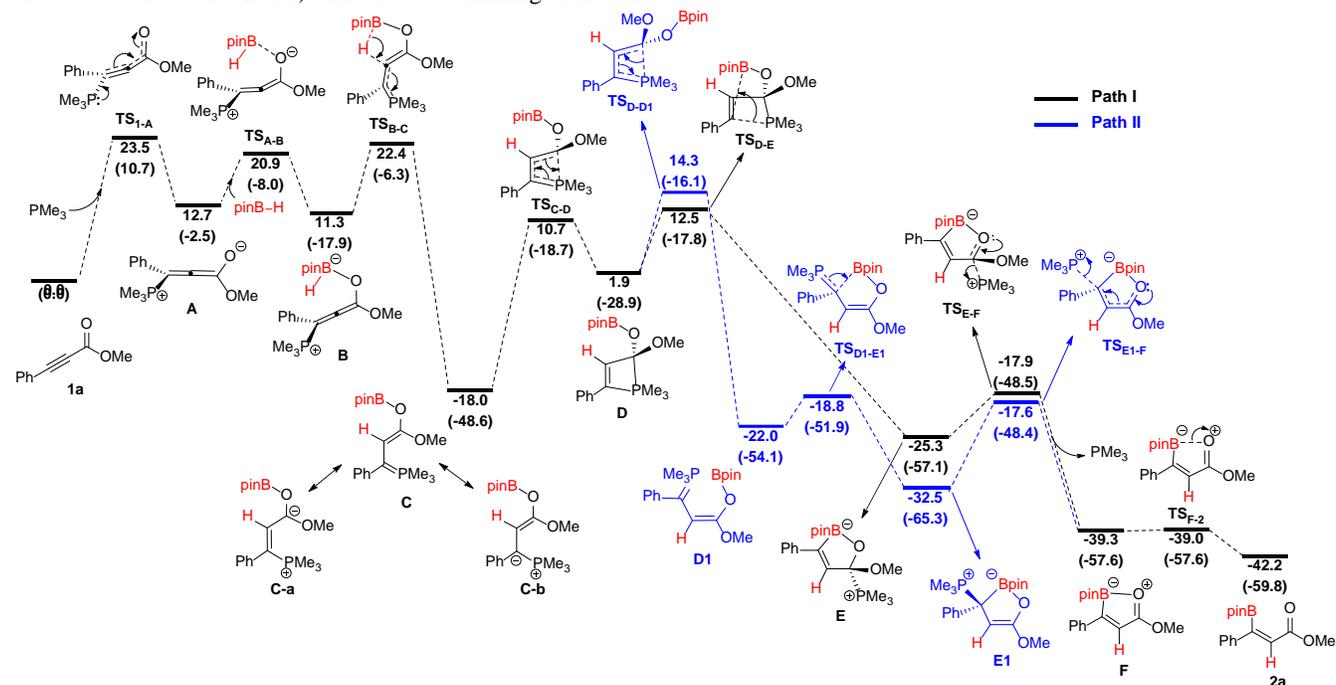
**Figure 1.** Energy profile calculated at B3LYP/6-31G\*\* for the proposed mechanism of *trans* hydroboration of methyl 3-phenylpropiolate. The solvation-corrected relative free energies and relative electronic energies (in parentheses) are given in kcal/mol.
