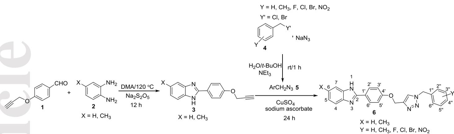
**Scheme 1.** Synthesis of benzimidazole-1,2,3-triazole hybrids **6**.
