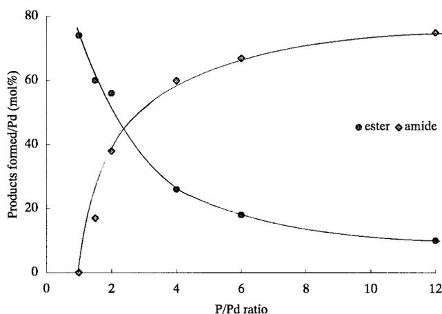
**Figure 1.** Effect of the PPh<sub>3</sub> ligands on the relative amounts of the ester and amide formed in reactions of 1:1 mixtures of Et<sub>2</sub>NH and EtOH with (phenylacetyl)palladium complexes
