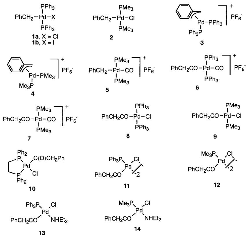
Analogue of **8** having  $\text{PMe}_3$  and dppe (dppe = 1,2-bis-(diphenylphosphino)ethane) ligands, **9** and **10**, were prepared by replacement of the  $\text{PPh}_3$  ligands in **8** with  $\text{PMe}_3$  and dppe ligands, respectively (see Experimental Section).
