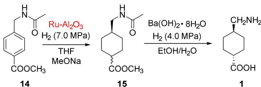
Based on the reported method of isomerization of *cis* isomer into *trans* isomer,<sup>4b</sup> we attempted to combine hydrolysis and isomerization of **15** in one step. The mixture of **15** and Ba(OH)<sub>2</sub> with ethanol and water as solvents was transformed smoothly to **1** at 250 °C and under hydrogen pressure of 4.0 MPa. After adjusting the pH value and clarification, **1** was obtained with 99.6% purity in 85.2% yield.
