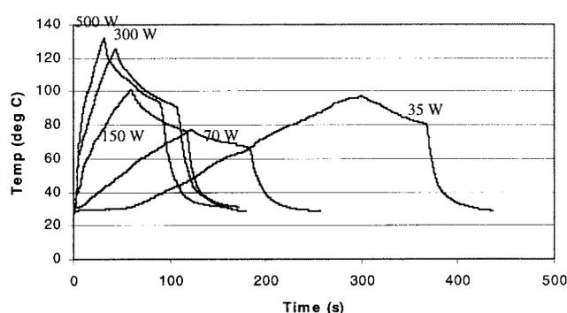
**Figure 2** The temperature of the reactions of 4-methoxyphenol in CH<sub>2</sub>Cl<sub>2</sub> were measured at the bottom of the reaction vessel
