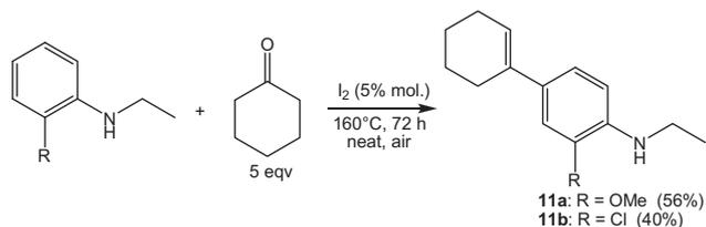
**Scheme 7.** Reaction between 2-chloro-*N*-ethylaniline or 2-methoxy-*N*-ethylaniline and cyclohexanone.
