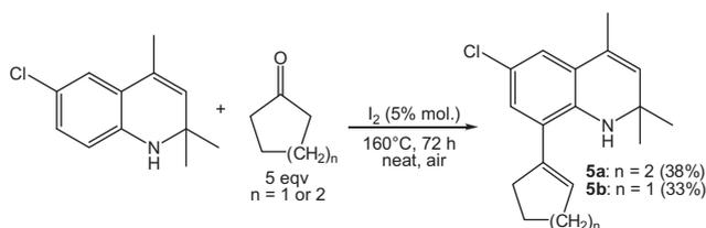
**Scheme 3.** Reaction between 6-chloro-1,2-dihydro-2,2,4-trimethylquinoline and cyclohexanone or cyclopentanone.
