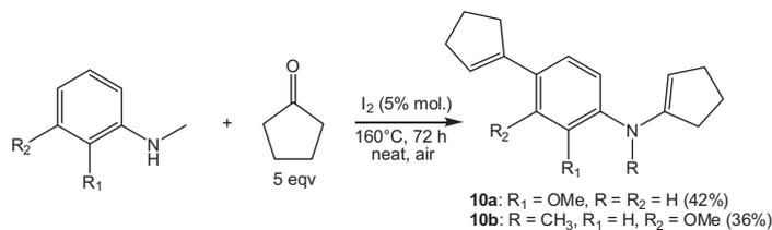
**Scheme 6.** Reaction between 2-methoxy-*N*-methylaniline or 3-methoxy-*N*-methylaniline and cyclopentanone.
