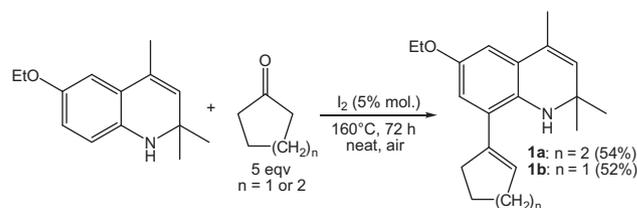
Scheme 1. Reaction between ethoxyquin and cyclohexanone or cyclopentanone.<sup>4a</sup>
