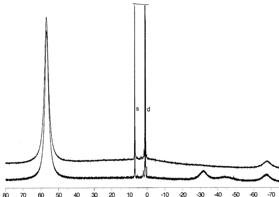
Figure 1. Proton NMR spectra (C<sub>6</sub>D<sub>6</sub> solutions, ppm values) of **10-d** (upper trace) and **10** (lower trace) (s = C<sub>6</sub>D<sub>5</sub>H, d = diamagnetic impurities)
