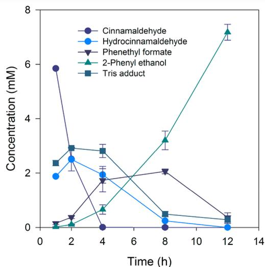
**Figure 3.** Time course of the conversion of cinnamaldehyde to 2-phenylethanol via the biocatalytic cascade reaction using formate dehydrogenase for cofactor regeneration. Conditions: 50 mM Tris-HCl buffer (pH 8), [ScOYE3] = 2  $\mu$ M, [BVMO<sub>AO</sub>] = 2  $\mu$ M, [CbFDH\_P2] = 0.2 U mL<sup>-1</sup>, [formate] = 50 mM, [NADP<sup>+</sup>] = 0.3 mM, [cinnamaldehyde] = 10 mM, *t* = 25 °C, shaking = 200 rpm.
