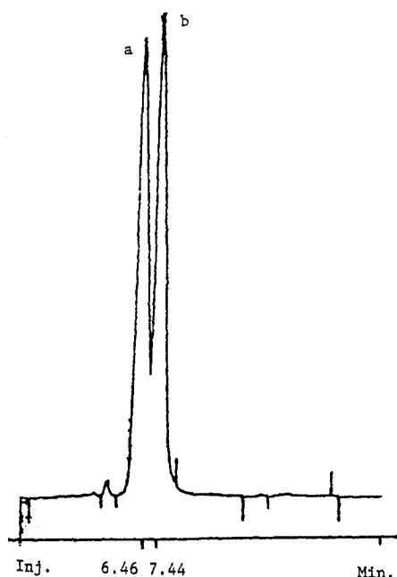
Figure 1. High-performance liquid chromatogram of diastereoisomeric mixture 8. Peaks: a = 8a; b = 8b. Column, Li-Chrosorb RP-18, 5 \mu m (250 \times 4.6 mm); mobile phase, H 2 O; flow-rate, 0.5 mL/min; absorption, 254 nm.
