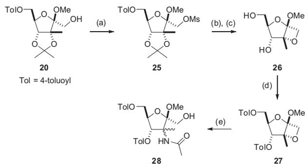
**Scheme 6.** Reagents and conditions: (a)  $\text{MsCl}$ ,  $\text{py}$ , rt, 18 h, 88%; (b)  $\text{TFA}/\text{H}_2\text{O}$  (9:1), rt, 0.5 h; (c)  $\text{NaOMe}$ ,  $\text{MeOH}$ , rt, 18 h; (d)  $p$ -toluoyl chloride,  $\text{py}$ , rt, 19 h, 46% (over 3 steps); (e) persilylated uracil,  $\text{MeCN}$ ,  $\text{SnCl}_4$ ,  $85^\circ\text{C}$ , 20 h, 30% (**28**).
