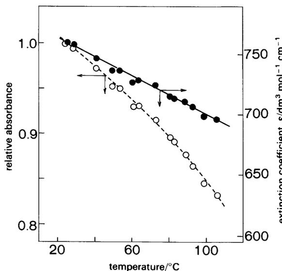
Fig. 3. Temperature dependence of  $\text{I}_2$  extinction coefficient,  $\epsilon$ , and relative absorbance. Total iodine as  $\text{I}_2 = 1.1 \times 10^{-3} \text{ mol dm}^{-3}$ ; path-length = 1.0 cm; wavelength = 460 nm.
