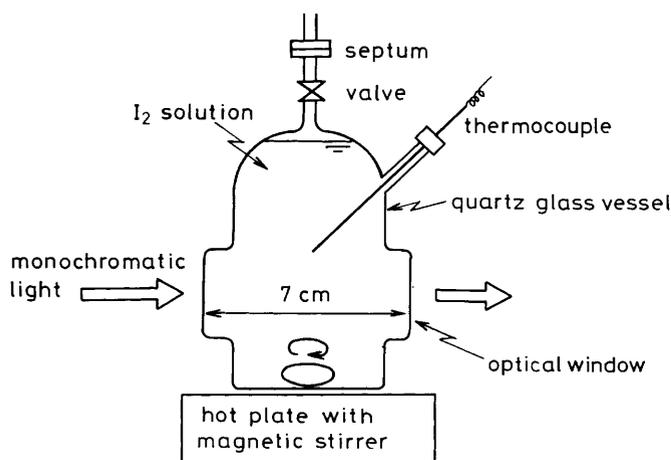
Fig. 2. Schematic view of sample cell.
