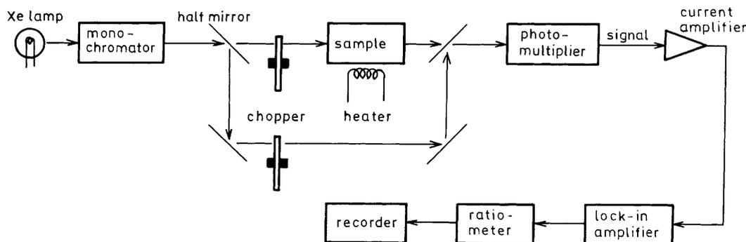
Fig. 1. Schematic diagram of spectrometer.
