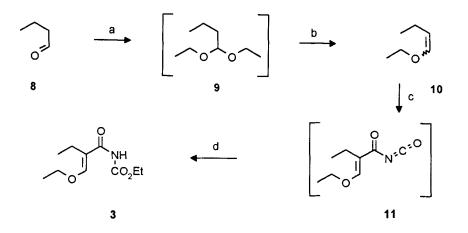
Reagents: (a) HC(OEt)<sub>3</sub>, NH<sub>4</sub>H<sub>2</sub>PO<sub>4</sub>, 60°C; (b) 140°C; (c) ClCONCO, dioxane, then Et<sub>3</sub>N; (d) EtOH.
