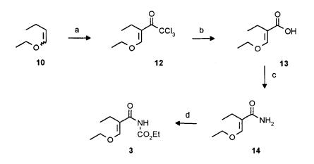
Reagents: (a) Cl<sub>3</sub>COCl, pyridine; (b) KOH, H<sub>2</sub>O, PhCH<sub>3</sub>; (c) (i) CDI, THF, (ii) NH<sub>3</sub>; (d) (i) LDA, THF, (ii) EtO<sub>2</sub>CCl.
