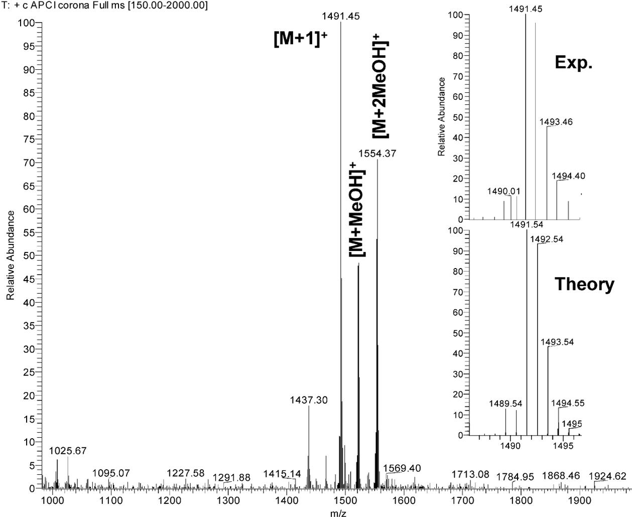
**Figure 4.** APCI MS of the iron(III) phthalocyanine-( $\mu$ -oxodimer) **4**.
