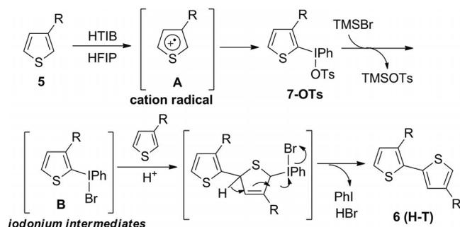
Scheme 5. Plausible mechanism for the coupling reaction.
