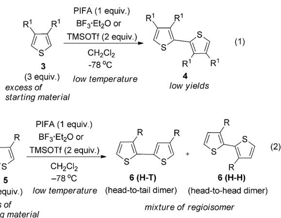
Scheme 2. Biaryl coupling reactions of 3-substituted thiophenes using hypervalent iodine reagent.
