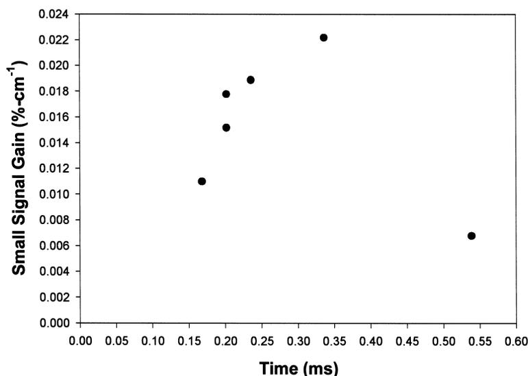
Fig. 4. The  $I(^2P_{3/2}) - I^*(^2P_{1/2})$  gain zone resulting from the  $NCl(a^1\Delta) + I(^2P_{3/2}) \rightarrow I^*(^2P_{1/2}) + NCl(X^3\Sigma)$  reaction. The gain profile extends over a reasonably long flow time of nearly 0.5 ms.
