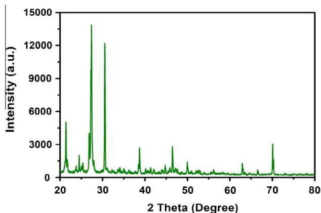
Fig. 6. X-ray diffraction of CPAT.
