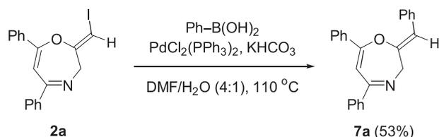
**Scheme 3.** Suzuki-Miyaura reaction of iodine-substituted 1,4-oxazepine **2a** with phenylboronic acid.
