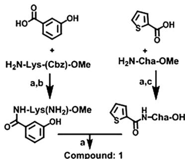
**Scheme 1.** General synthesis protocol for Compound **1**; *Reagents and conditions:* (a) EDC, HOBT, NMM, DMF, RT, overnight, (b)  $H_2/Pd/C$ , MeOH, RT, 6 h; (c) LiOH, MeOH:H<sub>2</sub>O (4:1), 5 h.
