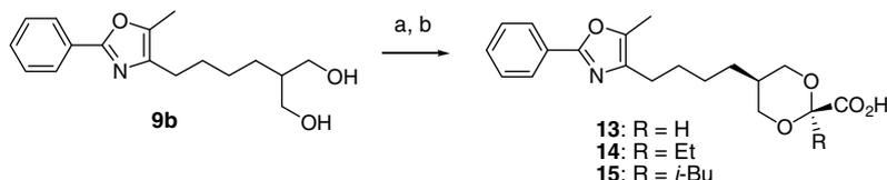
Scheme 2. Reagents: (a) i—RCOCO<sub>2</sub>Me, BF<sub>3</sub>·Et<sub>2</sub>O, MeCN, (b) aq NaOH, MeOH.
