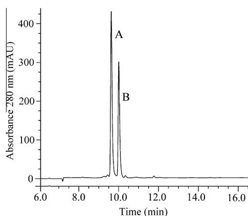
**Figure 2.** HPLC elution profile of the peptide H-Arg-Trp(Sar-Sar)-Ala-Arg-Tyr-Ala-OH exposed to pH 7.4 for 2 min at room temperature. The deprotected peptide H-Arg-Trp-Ala-Arg-Tyr-Ala-OH (B) shows an increased retention time indicating that the protected peptide (A) is more polar than the deprotected peptide (B).
