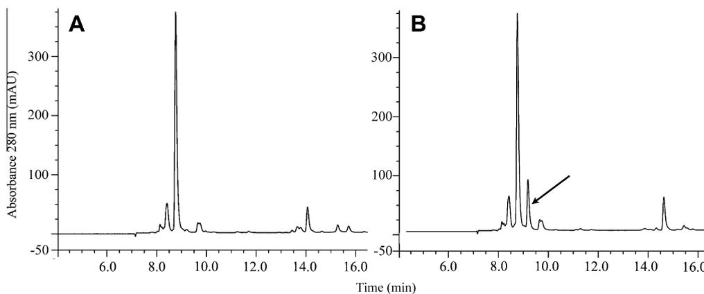
**Figure 1.** HPLC elution profile showing treatment of the peptide H-Arg-Trp(Sar-Sar)-Ala-Arg-Tyr-Ala-OH in 20% piperidine in NMP for 15 min (A), compared to treatment of the same peptide with 20% piperidine in NMP for 14 h and 40 min (B). The overnight treatment resulted in an additional peak (see arrow) corresponding to the deprotected product.
