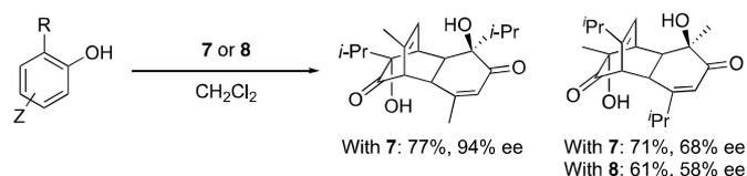
**SCHEME 1** The asymmetric hydroxylative dearomatization/[4+2]-dimerization cascade reactions of phenol derivatives mediated by chiral hypervalent iodine(V) reagents.
