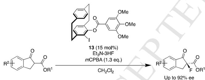
**SCHEME 2** Asymmetric fluorinations of  $\beta$ -ketoesters catalyzed by a planar chiral iodine reagent bearing a [2.2]paracyclophane unit.
