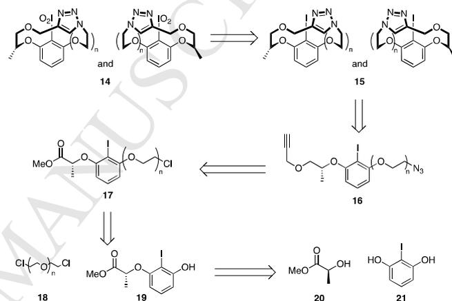
**SCHEME 4** Retrosynthesis of planar chiral hypervalent iodine(V) reagents bearing crown ether backbones.
