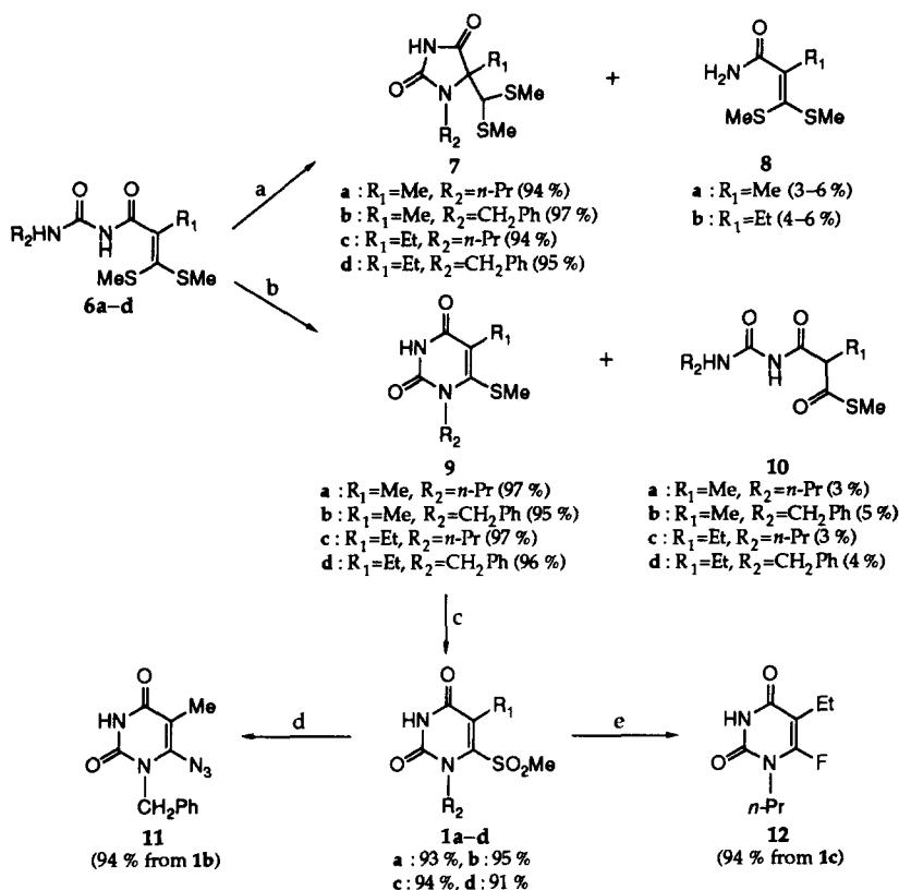
(a) K<sub>2</sub>CO<sub>3</sub> (2 eq.), EtOH, reflux, 0.5 h; (b) methanesulfonic acid (0.2 eq.), anhydrous AcOH, 80 °C, 3 h; (c) 3-chloroperoxybenzoic acid (5 eq.), benzene, reflux, 1 h; (d) NaN<sub>3</sub> (1 eq.), DMF, rt, 0.5 h; (e) (*n*-Bu)<sub>4</sub>NF (3 eq.), THF, reflux, 0.5 h
