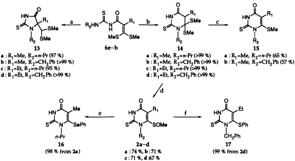
(a) K<sub>2</sub>CO<sub>3</sub> (2 eq.), EtOH, reflux, 0.5 h; (b) methanesulfonic acid (0.2 eq.), anhydrous AcOH, rt, 15 min; (c) methanesulfonic acid (0.2 eq.), anhydrous AcOH, 120 °C (bath temp.), 22 h; (d) NaIO<sub>4</sub> (6 eq.), H<sub>2</sub>O, MeOH, reflux, 0.5 h; (e) PhSeH (3 eq.), NaOH, EtOH, rt, 16 h; (f) PhSH (1 eq.), NaOH, EtOH, rt, 16 h
