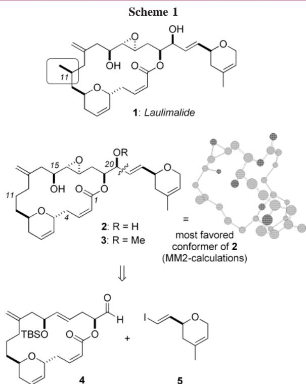
iodide **5**. Notably, this synthesis design should enable the modular construction of a wide range of laulimalide analogues with unnatural side chains.
