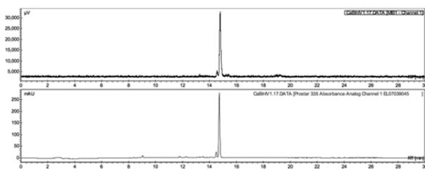
**Figure 2.** HPLC chromatograms of [ $^{125}\text{I}$ ]11a coinjected with the reference standard 11a. Radiochromatogram (upper trace) and UV-visible ( $\lambda = 254 \text{ nm}$ ) chromatogram (lower trace) are shown.
