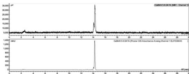
**Figure 3.** Radiochromatogram (upper trace) and UV-visible ( $\lambda = 254 \text{ nm}$ ) HPLC chromatogram (lower trace) of [ $^{125}\text{I}$ ]23a coinjected with the reference standard 23a.
