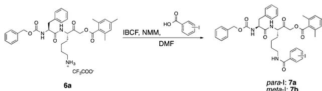
desired products **7a** and **7b** were isolated following simple extraction in yields of 29% and 45%, respectively. To generate the ureas, **6a** was combined with 3- or 4-iodophenyl isocyanate in the presence of triethylamine, giving **8a** and **8b** in 9% and 14% yields, respectively, following silica gel chromatography (Scheme 2).
