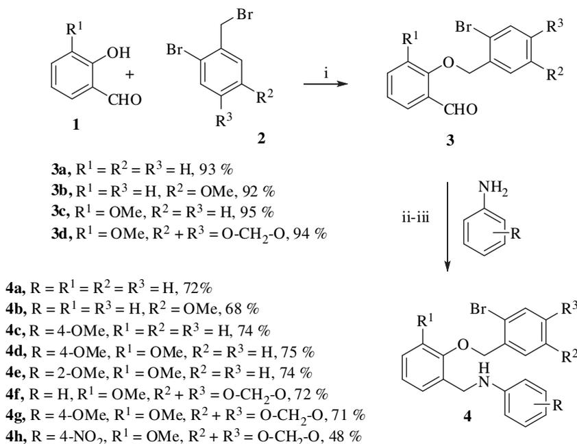
**Scheme 1.** Synthesis of O-bromobenzylated aromatic amines. Reagents and conditions: (i) acetone, K<sub>2</sub>CO<sub>3</sub>, reflux, 3 h (ii) EtOH, 25 °C, 12 h (iii) NaBH<sub>4</sub>, EtOH, 0 °C, 2 h.
