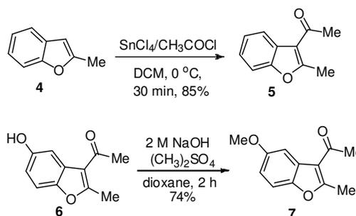
Scheme 1. Synthesis of 2-acetyl-3-methylbenzofurans **5** and **7**.
