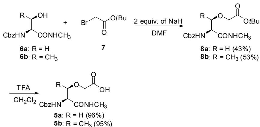
**Scheme 3.** Preparation of **5a,b** from **6a,b**.
