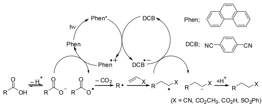
**Scheme 2.** Photoinduced decarboxylative radical addition of carboxylic acids to electron-deficient alkenes.
