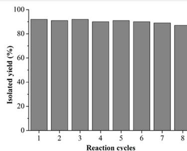
Figure 2 Recycling of the 2P-MCM-41-Pd(OAc)<sub>2</sub> complex
