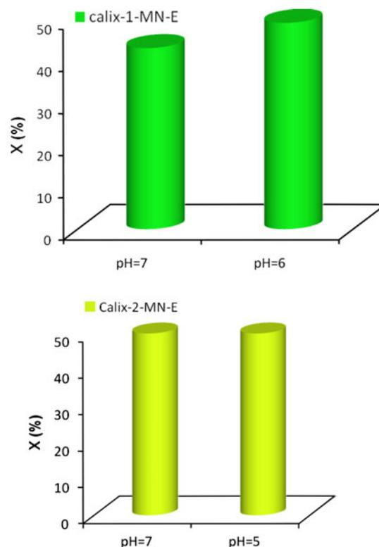
**Fig. 8** Effect of pH on the conversion (x) in the hydrolysis of racemic naproxen methyl ester with **Calix-1-MN-E** and **Calix-2-MN-E**
