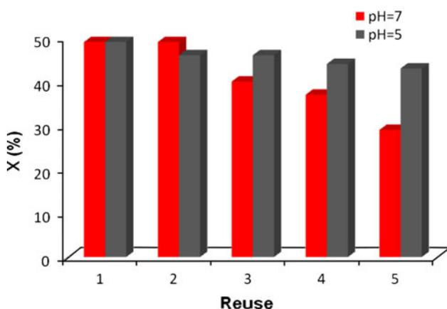
**Fig. 10** Reusability on the conversion (x) in the hydrolysis of racemic Naproxen methyl ester with **Calix-2-MN-E** for different pH
