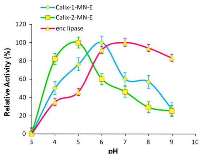
**Fig. 6** Effect of substrate pH on residual activity of encapsulated lipases
