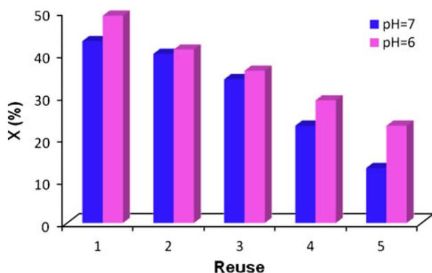
**Fig. 9** Reusability on the conversion (x) in the hydrolysis of racemic Naproxen methyl ester with **Calix-1-MN-E** for different pH
