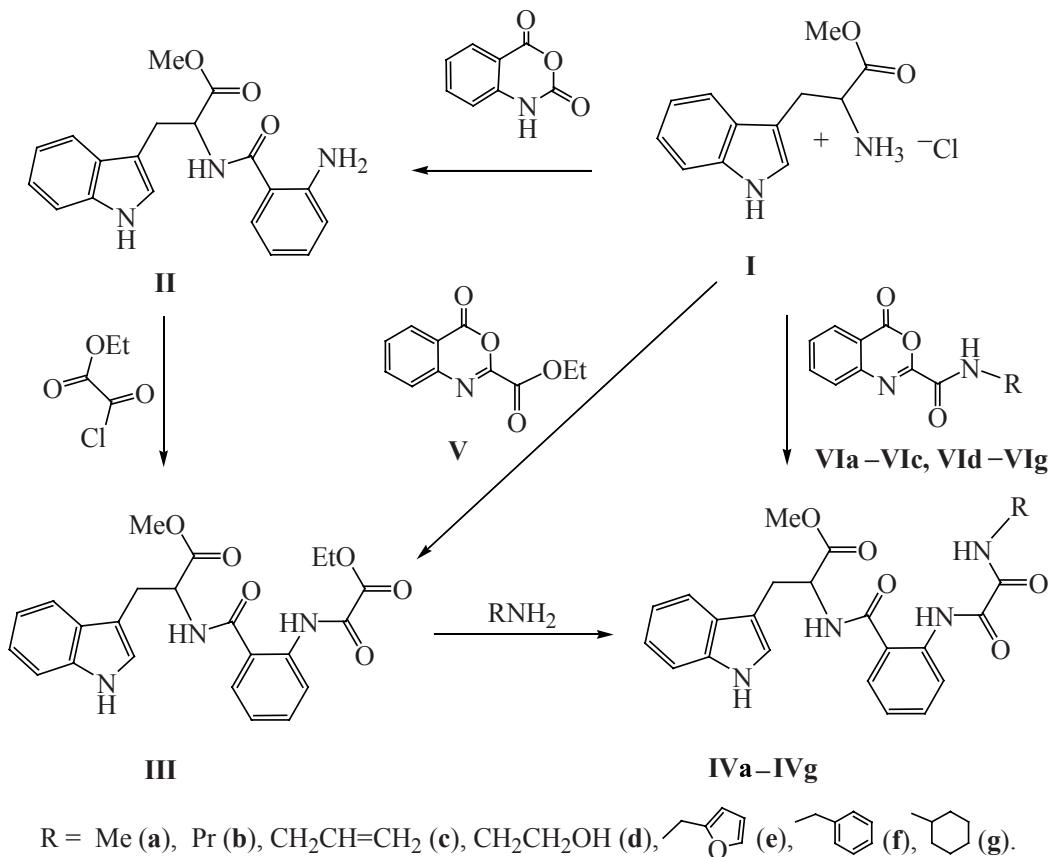
and aromatic amines they form *N*-(R-substituted) amides of 4-oxo-3,4-dihydroquinazoline-2-carboxylic acid [11]. However the acylation of ester **I** with 3,1-benzoxazine **V** even at boiling the reaction mixture gave only compound **III**, most likely because of considerable steric hindrances at the benzamide moiety of molecule **II**.
