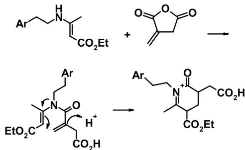
Figure 3. Anhydride addition to  $\beta$ -enamine.
