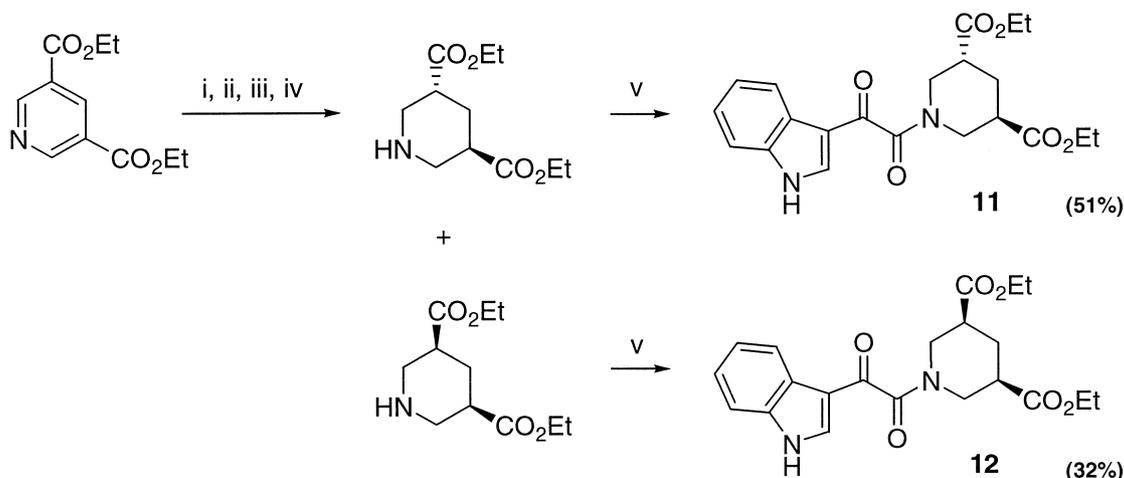
**Scheme 3.** Reagents and conditions: (i)  $\text{H}_2$ ,  $\text{PtO}_2$ ,  $\text{AcOH}$  (58%); (ii)  $\text{BOC}_2\text{O}$ ,  $\text{Et}_3\text{N}$ ,  $\text{CH}_2\text{Cl}_2$ , rt (87%); (iii) silica chromatography; (iv)  $\text{HCl}$ ,  $\text{EtOAc}$ , rt (100%); (v) indole-3-glyoxylyl chloride,  $\text{Et}_3\text{N}$ ,  $\text{MeCN}$ , rt.
