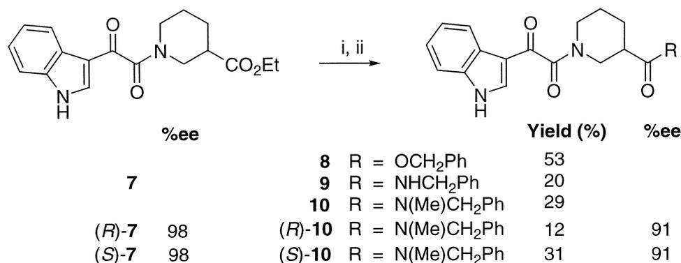
Scheme 2. Reagents and conditions: (i) LiOH, THF-H<sub>2</sub>O, rt (76–93%); (ii) CDI, ROH, Et<sub>3</sub>N, THF, rt or BOPCl, Et<sub>3</sub>N, NHR<sup>2</sup>R<sup>3</sup>, CH<sub>2</sub>Cl<sub>2</sub>, rt.
