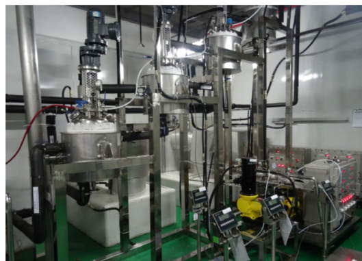
Figure 5. In-series CSTR used in the continuous process.
