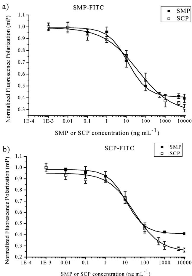
**Figure 4.** FPIA calibration curves for SMP and SCP using the same MAb and two different tracers: (a) SMP-FITC and (b) SCP-FITC. FPIA calibration curve and the SCP and SMP standard drug were dissolved in BB buffer. FP values, which are means of three replicates, were plotted against analyte concentration.
