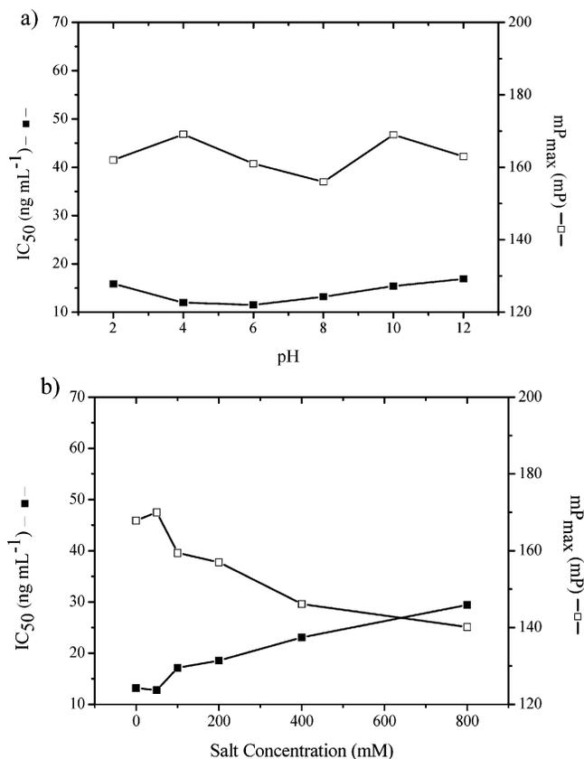
**Figure 5.** Influence of the (a) pH and (b) salt concentration of assay buffer on the analytical characteristics of SMP competitive standard curve: (■) value of  $IC_{50}$  for SMP and (□)  $mP_{max}$  value in the absence of SMP ( $mP_{max}$ ). All reagents were prepared in BB at the appropriate pH and salt concentration. Each point represents the mean of three replicates.
