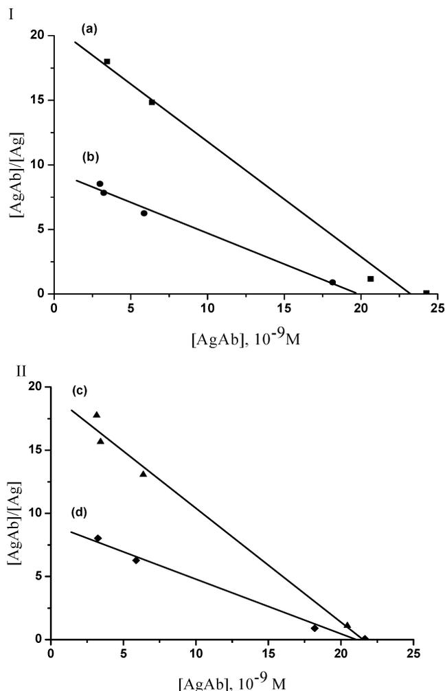
**Figure 7.** Scatchard plot for  $K_{aff}$  calculation. I: (a) tracer SCP-FITC, antigen SMP,  $Y = -0.903X + 19.442$ ; (b) tracer SCP-FITC, antigen SCP,  $Y = -0.433X + 9.121$ . II: (c) tracer SMP-FITC, antigen SMP,  $Y = -0.891X + 20.716$ ; (d) tracer SMP-FITC, antigen SCP,  $Y = -0.478X + 9.488$ .
