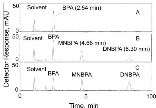
**Fig. 2.** Typical RP-HPLC chromatograms of the reaction mixtures in which BPA (initial concentration: 200  $\mu$ M) was allowed to react with (A) 0, (B) 200, or (C) 500  $\mu$ M peroxyxynitrite in 2.0 mL of 0.08 M phosphate buffer, pH 7.0 that also contained 0.1 mM DTPA and 0.01 M NaHCO<sub>3</sub>. Aliquots (20  $\mu$ L each) of the reaction mixture were analyzed as described in Section 2.
