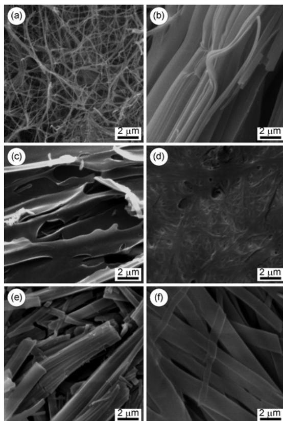
**Figure 1** SEM images of the xerogels from the gels of **1**/benzene (a), **2**/benzene (b), and **3**/benzene (c) and those from **1**/1-heptanol (d), **2**/1-heptanol (e), and **3**/1-heptanol (f).
