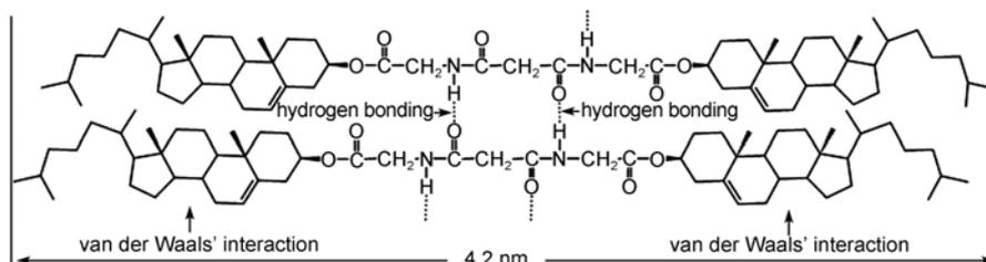
Figure 7 A possible aggregation mode of gelator **2** in benzene.
