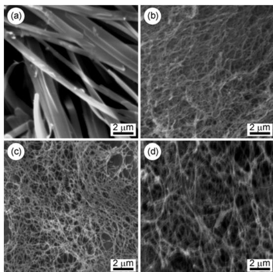
**Figure 3** SEM images of the xerogels of **2** from cyclohexane at different concentrations. (1) 3.0%; (2) 2.0%; (3) 1.0%; (4) 0.5%.
