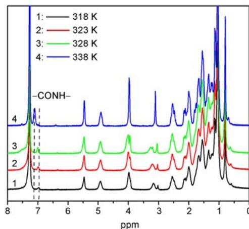
**Figure 5** Temperature-dependent  $^1\text{H}$  NMR spectra of **2**/benzene gel.
