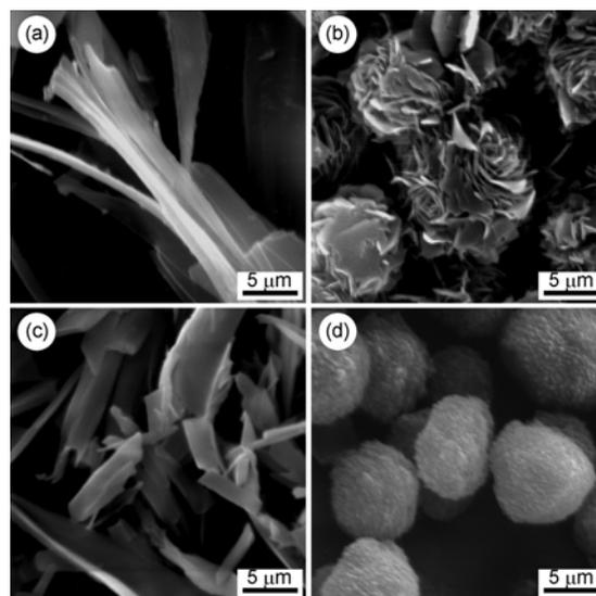
**Figure 2** SEM images of the xerogels of **2** (a) and **4** (c) from DMSO and those of the precipitates of **3** (b) and **5** (d) from the same solvent.
