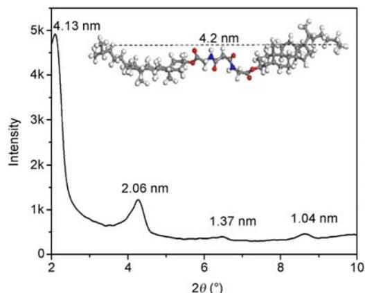
Figure 6 X-ray diffraction trace of the fresh gel of **2**/benzene (3%).
