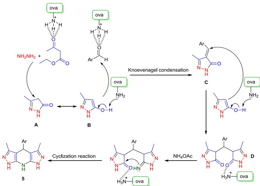
Scheme 2 Plausible mechanism for synthesis of tetrahydropyrazolo pyridine derivatives in the presence of nano-ovalbumin
