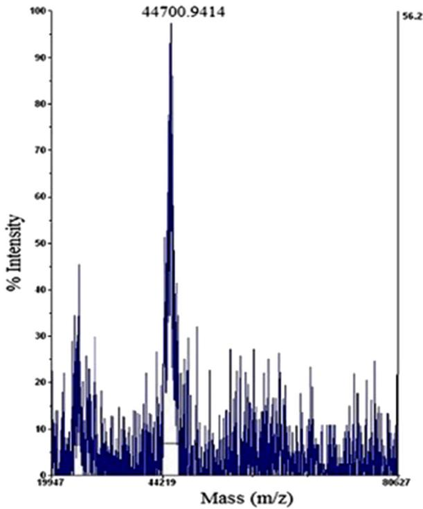
Fig. 5 MALDI-TOF/TOF mass spectrum of nano-ovalbumin (0.016 g of ovalbumin was dissolved in 0.5 mL of 7.0 M aqueous solution of guanidinium chloride)
