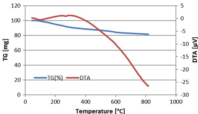
**Fig. 6** Thermal gravimetric analysis (TGA/DTA) pattern of nano-ovalbumin
