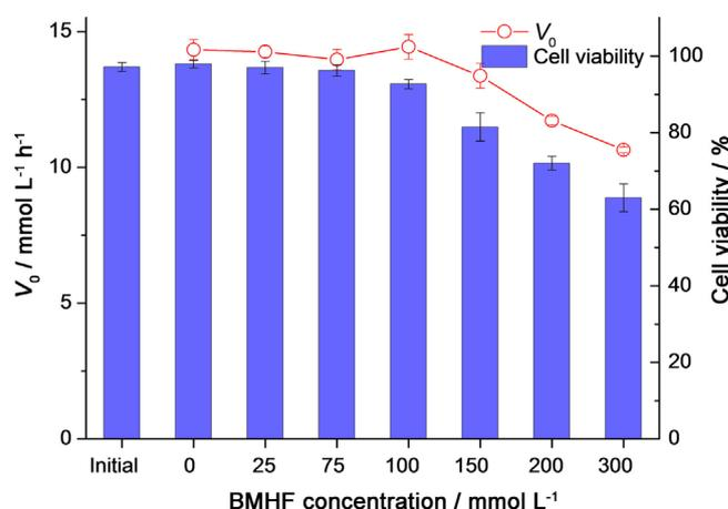
**Figure 4.** Effect of the product concentrations of BHMF synthesis and cell viability. Conditions: 50 mM HMF, 30 mM glucose, BHMF of the designated concentration, 20 mg mL<sup>-1</sup> microbial cells, 4 mL phosphate buffer (100 mM, pH 7.2), 200 rpm, 35 °C; after microbial cells were incubated for 12 h under the above conditions without HMF, cell viability was measured.
