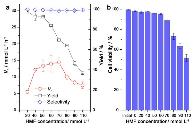
**Figure 2.** Effects of substrate concentrations on a) BHMf synthesis and b) cell viability. Reaction conditions: 30 mM glucose, 20 mg mL<sup>-1</sup> microbial cells, 4 mL phosphate buffer (100 mM, pH 7.2), 200 rpm, 35 °C; a) reaction periods: 5, 7, 7, 12, 24, 36, 12 and 7 h, with gradually increasing HMF concentrations from 20 to 110 mM, respectively; b) incubation period of 12 h.
