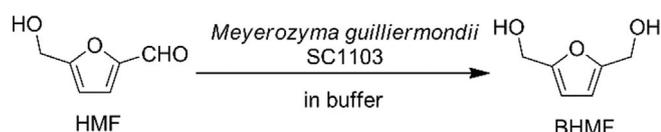
Scheme 1. Biotransformation of HMF to BHMf in buffer.
