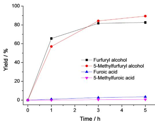
**Figure 6.** Biocatalytic reduction of furfurals to furfuryl alcohols. Reaction conditions: 50 mM furfurals, 30 mM glucose, 20 mg mL<sup>-1</sup> microbial cells, 4 mL phosphate buffer (100 mM, pH 7.2), 200 rpm, 35 °C.
