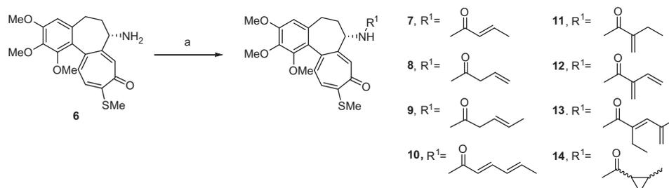
**Scheme 1.** Reagents and conditions: (a) carboxylic acids, EDC,  $\text{CH}_2\text{Cl}_2$ , rt, **7**: 92%, **8**: 96%, **9**: 78%, **10**: 62%, **11**: 63%, **12**: 53%, **13**: 71%, **14**: 98%.
