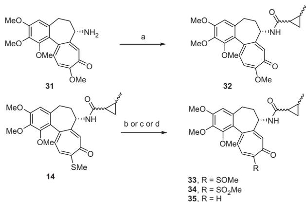
**Scheme 4.** Reagents and conditions: (a) 2-methylcyclopropanecarboxylic acid, EDC, CH<sub>2</sub>Cl<sub>2</sub>, rt, 71%; (b) R = SOMe:*m*CPBA (1.05 equiv), CH<sub>2</sub>Cl<sub>2</sub>, rt, 82%; (c) R = SO<sub>2</sub>Me:*m*CPBA (2.5 equiv), CH<sub>2</sub>Cl<sub>2</sub>, rt, 84%; (d) R = H, (i) Raney Ni, EtOH, rt, 70%, (ii) Pd/C, toluene, reflux, 31%.
