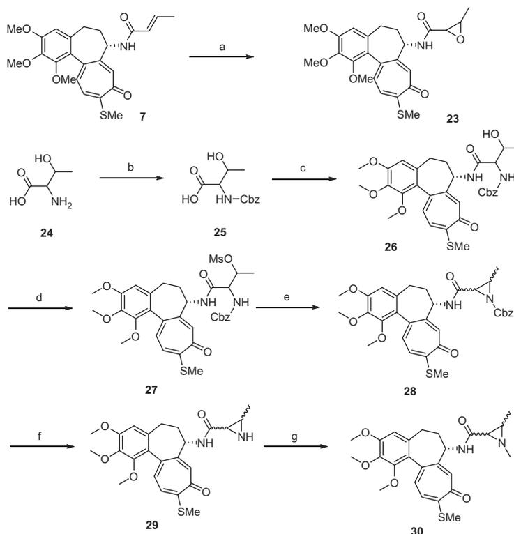
**Scheme 3.** Reaction conditions and reagents: (a) *m*CPBA, CH<sub>2</sub>Cl<sub>2</sub>, rt, 82%; (b) CbzCl, NaHCO<sub>3</sub>, THF, water, rt, 93%; (c) **6**, EEDQ, Et<sub>3</sub>N, CH<sub>3</sub>CN, 48%; (d) MsCl, Et<sub>3</sub>N, CH<sub>2</sub>Cl<sub>2</sub>, rt, quant.; (e) *t*-BuOK, *t*-BuOH, CH<sub>2</sub>Cl<sub>2</sub>, 0 °C to rt, 38%; (f) KOH, THF, water, rt, 9%; (g) MeI, K<sub>2</sub>CO<sub>3</sub>, MeOH, 50 °C, 65%. EEDQ = *N*-ethoxycarbonyl-2-ethoxy-1,2-dihydroquinoline.
