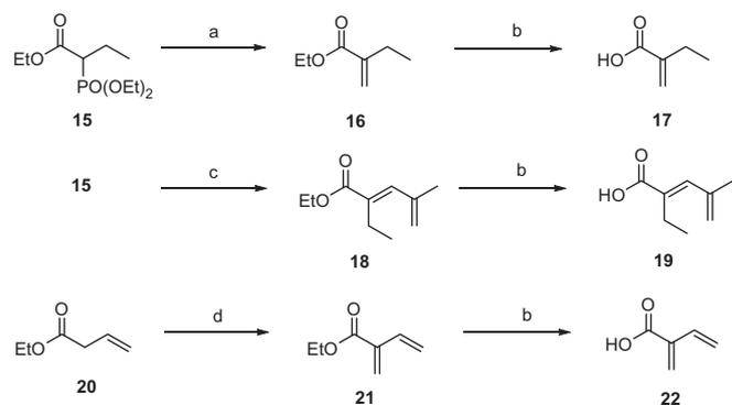
**Scheme 2.** Reagents and conditions: (a)  $(\text{CH}_2\text{O})_n$ , NaH, DMF, rt, 66%; (b) NaOH, MeOH,  $\text{H}_2\text{O}$ , rt, **17**: 83%, **19**: 78%, **22**: 69%; (c) methacrolein, NaH, DMSO, rt, 91%; (d)  $(\text{CH}_2\text{O})_n$ , NaH, DMF, rt, 91%.
