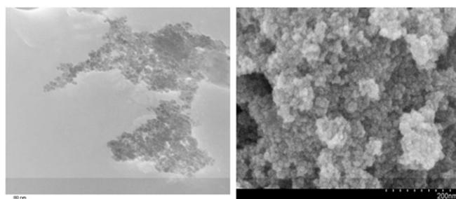
**Figure 11.** TEM and SEM images of reused catalyst after five runs.
