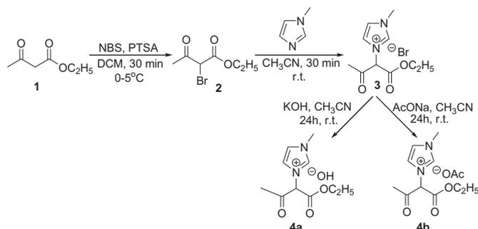
Scheme 1. Synthesis of ethylacetoacetate tagged imidazolium IL 4a and 4b.
