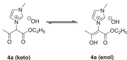
Fig. 1. The coexistence of keto and enol forms of ethylacetoacetate tagged imidazolium hydroxide 4a.
