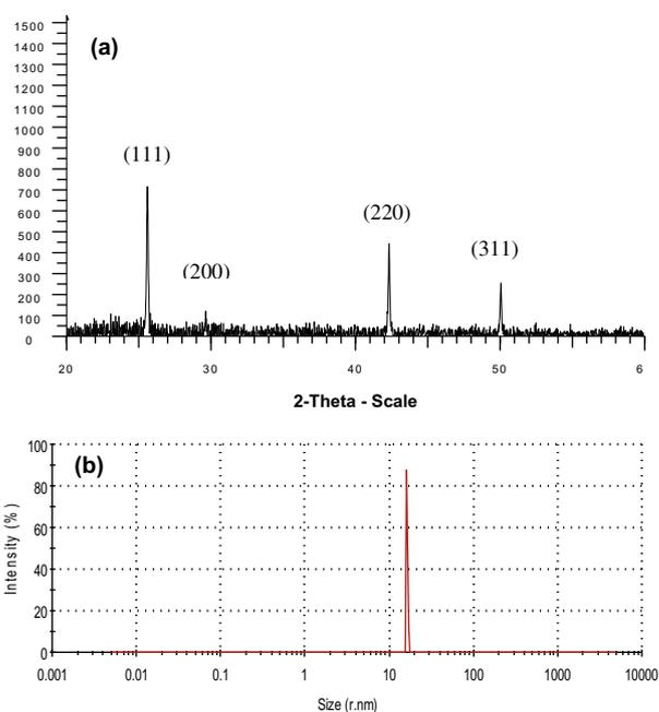
Fig. 2. Characterization of CuI nanoparticles (a) XRD image (b) DLS showing intensity distributed particle size (c) SEM image (d) TEM image.
