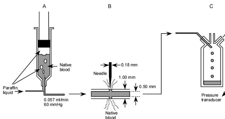
Fig. 2. Principle of Haemostatometry
