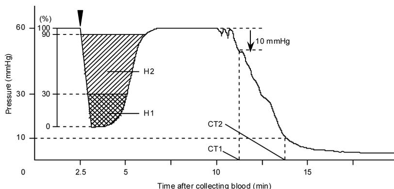
Fig. 3. A Typical Haemostatograph
