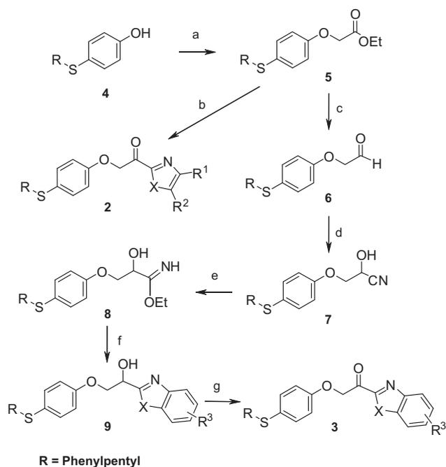
**Scheme 1.** Reagents and conditions: (a) ethyl bromoacetate,  $\text{Cs}_2\text{CO}_3$ , DMF, rt, 88%; (b) 2-lithiated heterocycle, THF,  $-78^\circ\text{C}$  to rt, 50–80%; (c)  $\text{dibal}$ , THF,  $-78^\circ\text{C}$  to rt, 83%; (d) acetonecyanohydrin, TEA, rt, 60%; (e) HCl, EtOH, rt, >95%; (f) 1,2-diaminobenzene or 2-aminophenol, MeCN, reflux, 45–70%; (g) Dess–Martin reagent, rt, 50–70%.
