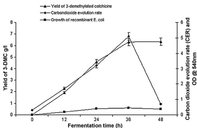
**Fig. 7.** Relationship between carbon dioxide evolution rate (CER), *E. coli* growth rate and bioconversion yield of colchicine into their derivatives at 70 l bioreactor.
