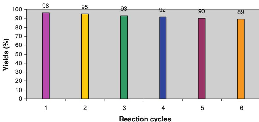
**Fig. 2** Recycling of nano  $\text{TiO}_2\text{-HClO}_4$  as catalyst in the preparation of methyl (4-chlorophenyl)(2-hydroxynaphthalen-1-yl)methyl carbamate
