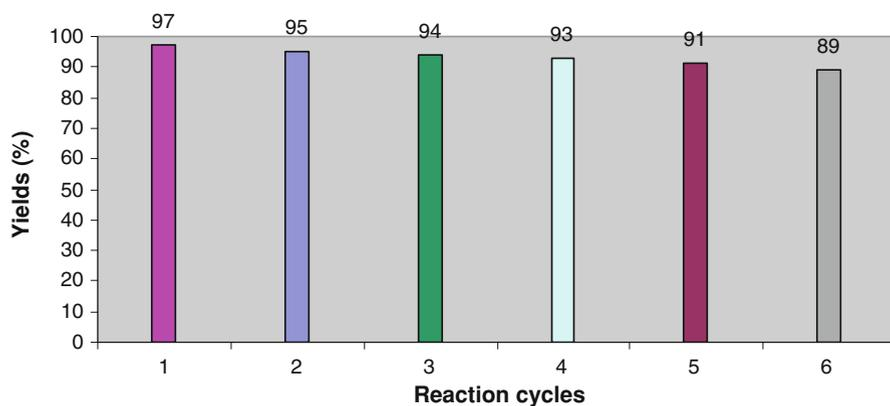
**Fig. 1** Recycling of nano TiO<sub>2</sub>-HClO<sub>4</sub> as catalyst in the preparation of *N*-[(4-chlorophenyl)-(2-hydroxynaphthalen-1-yl)methyl]acetamide
