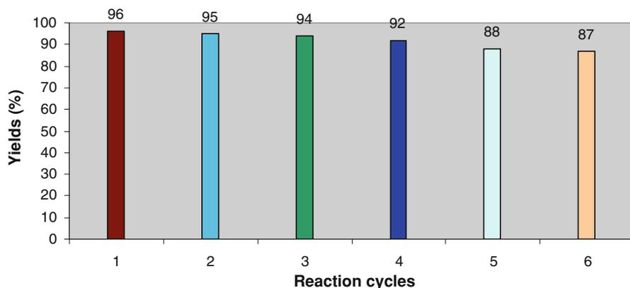
**Fig. 3** Recycling of nano TiO<sub>2</sub>-HClO<sub>4</sub> as catalyst in the preparation of 1-((4-chlorophenyl)(piperidin-1-yl)methyl)naphthalen-2-ol
