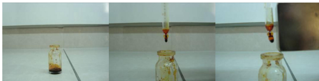
Fig. 1. Image of the [\text{C}_2\text{OHmim}]\text{FeCl}_3\text{Br}^- ionic liquid droplet attracted toward a NbFeB magnet.
