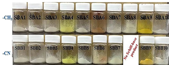
FIGURE 5 Photos of the 20 target Schiff bases, abbreviated as SBA1–SBA10 and SBB1–SBB10 , obtained from a solvent-free mechanochemical reaction between 10 differently functionalized aromatic aldehydes with p -toluidine and with 4-aminobenzonitrile
