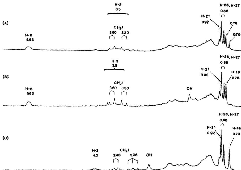
Figure 3. Proton nuclear magnetic resonance spectra. Chemical shifts are given in ppm from TMS. (A) Compound I, prepared by the method of reference (1). (B) Compound I, prepared by the method of reference (7). (C) Compound II.
