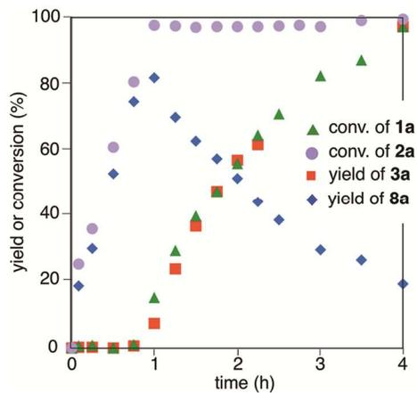
**Figure 3.** Time-course of the sulfenylation of **1a** (0.2 M) with **2a** (1.2 equiv) carried out in  $CH_3CN$  in the presence of **5a•TfO** (2 mol%) and  $I_2$  (4 mol%) under molecular oxygen (1 atm) at 50 °C.
